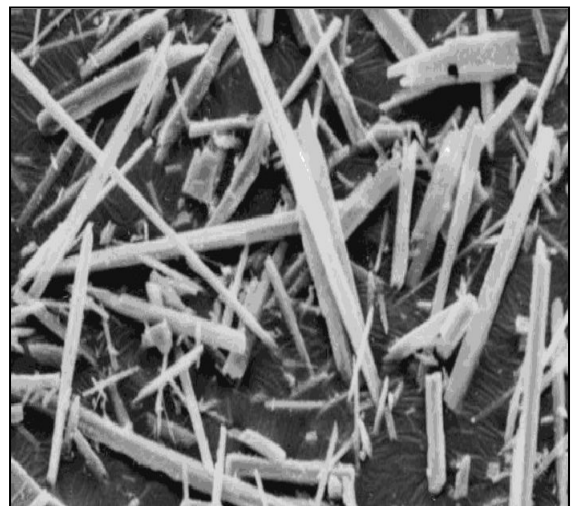
TREMIN ® 939 wollastonite, Quarzwerke GmbH chem. formula CaSiO_3 distinct needle structure
