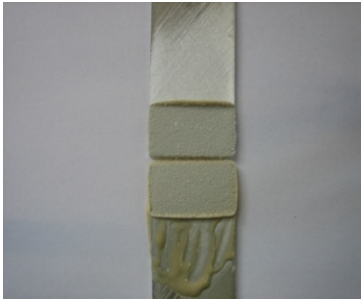
Cohesion breakage of the formulation with Calcium Carbonate
