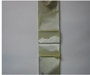
Uniform adhesion breakage of the formulation with TREMIN® 939-600 AST
